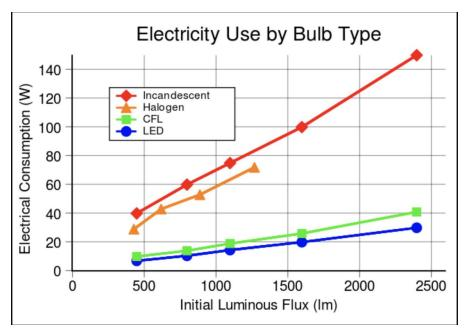
This graph shows how efficient the different kinds of light bulbs are. As we can see, incandescent bulbs are the most inefficient of the bulbs in the chart whereas LED lights are the most efficient of the ones being compared. This means that by using LED lights, we can save energy and therefore the money that energy costs.
